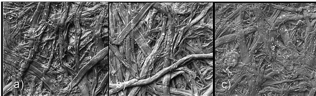
Fig. 4. SEM observation on the surface structure of paper folios A, B, and C at 500× magnification.
