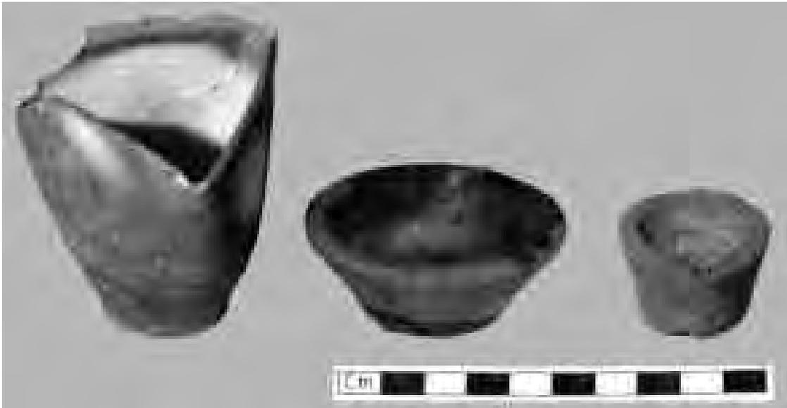
FIG. 1 – From left to right: triangular crucible, scorifier and bone-ash cupel, the basic set of equipment in a fire assay laboratory. Scale bar is 10 cm.
