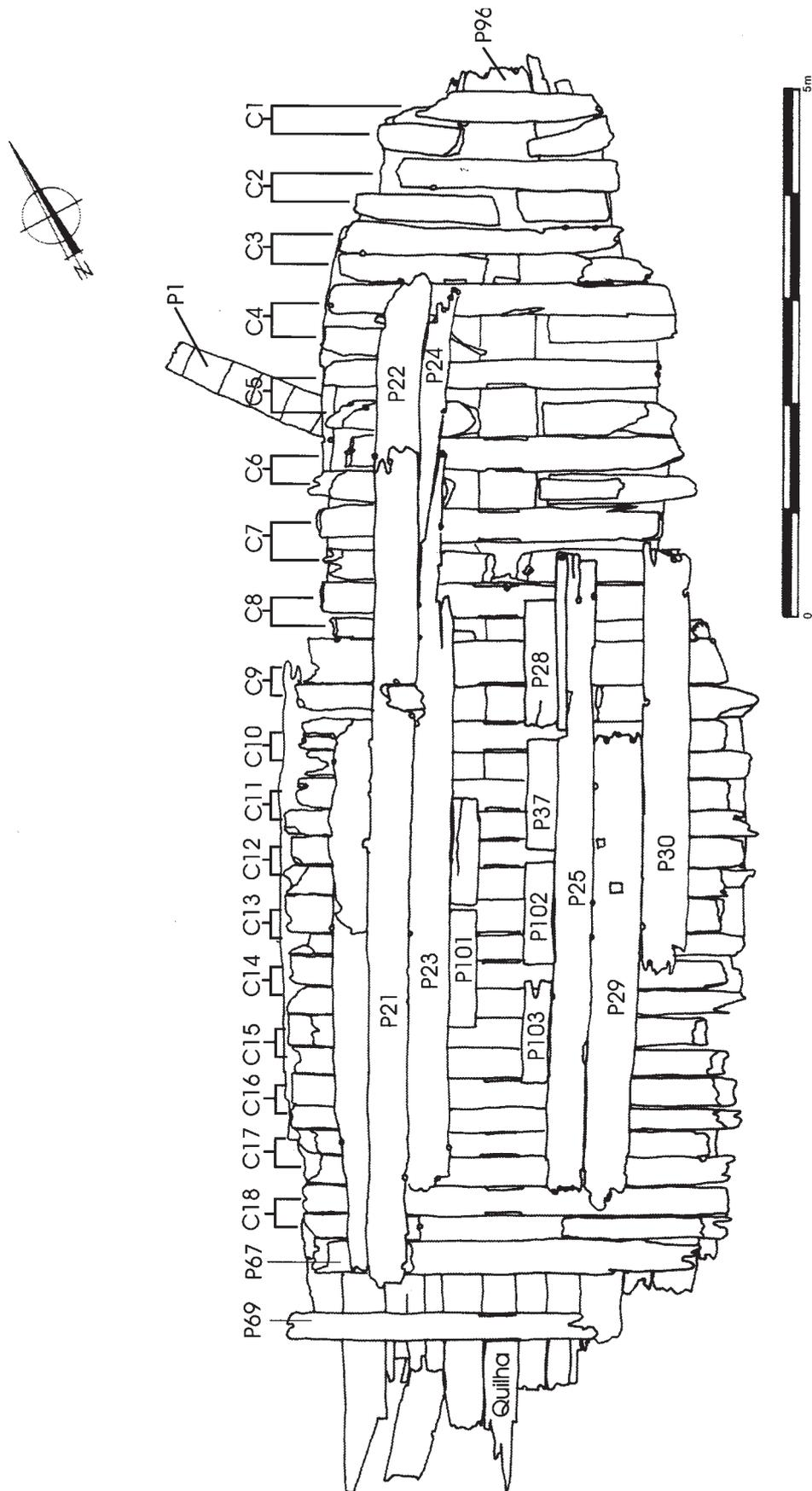
FIG. 1 – Angra C plan of the hull.
