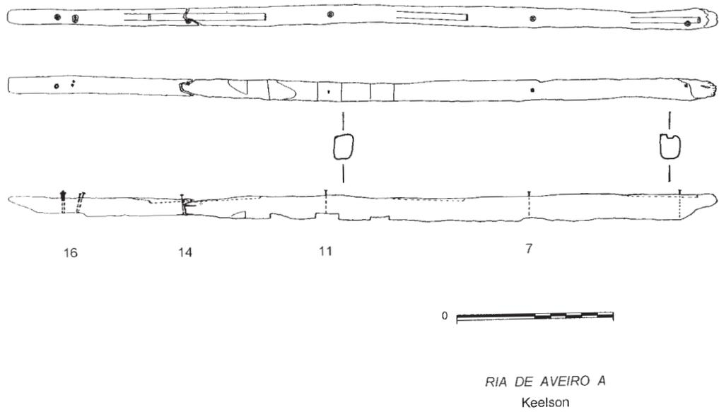
FIG. 17 – Drawing of the preserved parts of the keelson of the Ria de Aveiro A shipwreck.
