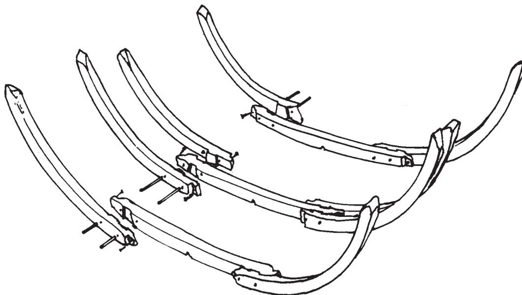
FIG. 10 – Scheme of the typical central framing pattern in the medieval and post-medieval Mediterranean and Iberian-Atlantic shipbuilding traditions.
