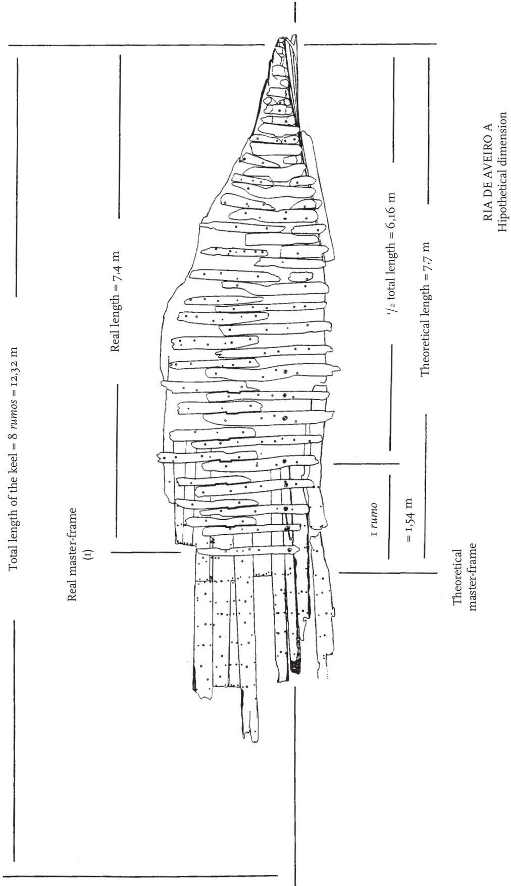
FIG. 11 – Dimensions of the Ria de Aveiro A shipwreck.
