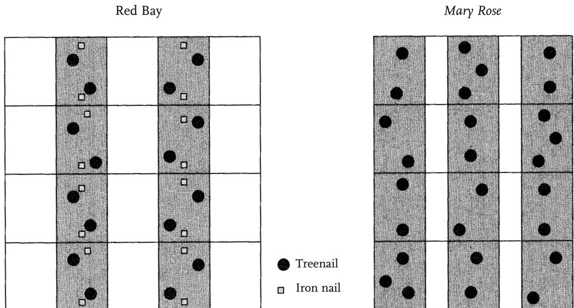
FIG. 10 – The typical arrangement of treenails and iron nails holding the hull planks.
