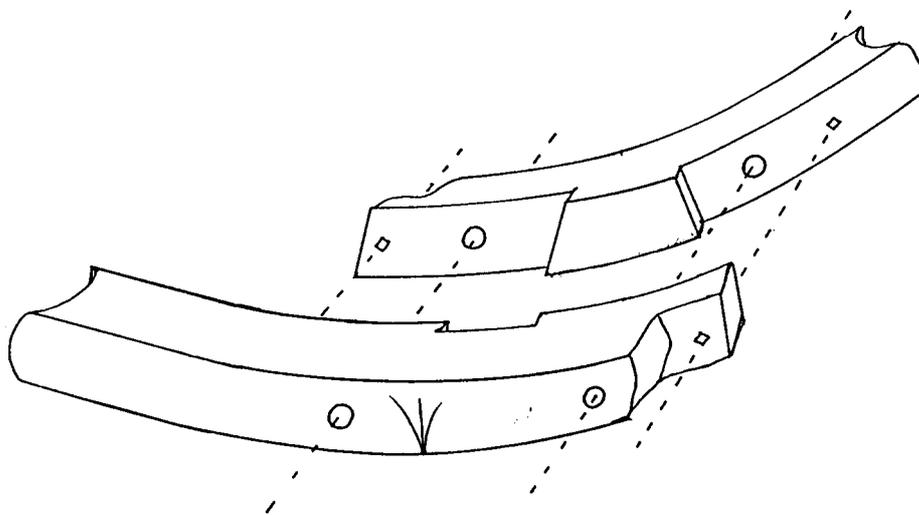
FIG. 6 – The “dovetail mortice” feature linking the floor timber and the first futtock, showing the round treenails and the square nails typically found in Biscayan wrecks.
