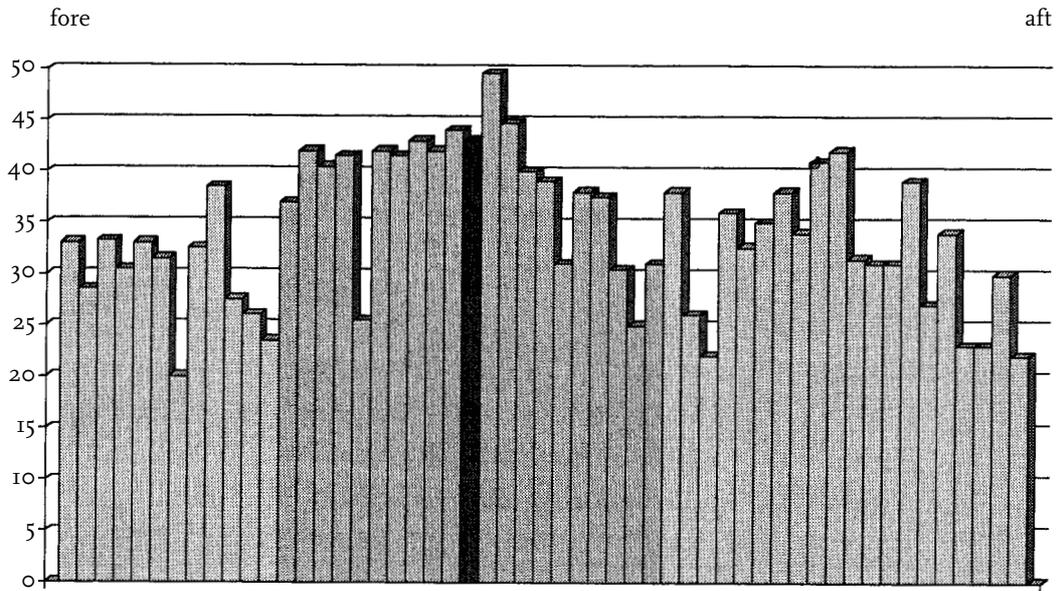
FIG. 9 – The sided dimension, or room, of the *Mary Rose* floor timbers at the keel (cm).
