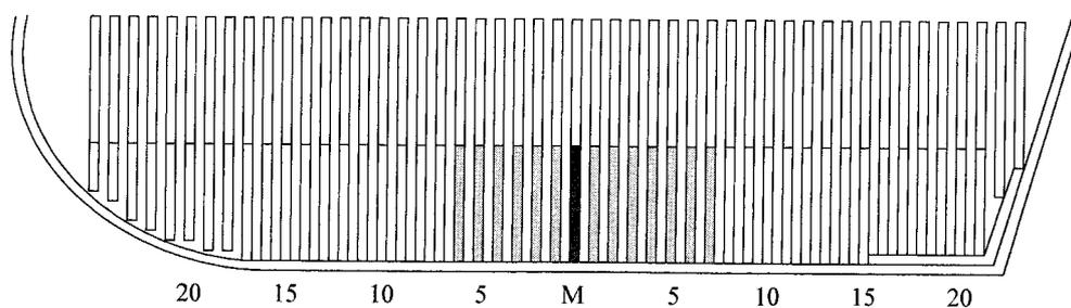
FIG. 5 – The positions of mortices frames in the *Mary Rose* and the Red Bay ship.
