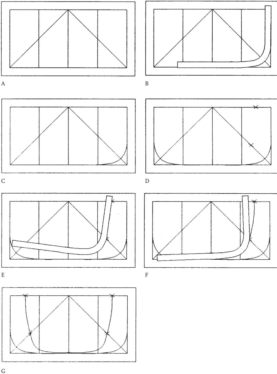
FIG. 9 – Diagram to illustrate the design of *vattai* frames using a scribe board and a single mould. Drawing: E. Kentley
