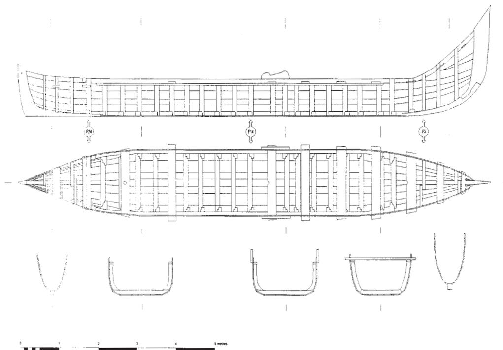
FIG. 6 – Rectified plans of a *vattai* recorded on the Eripurakarai foreshore in January, 1997. Drawing: E. Kentley.
