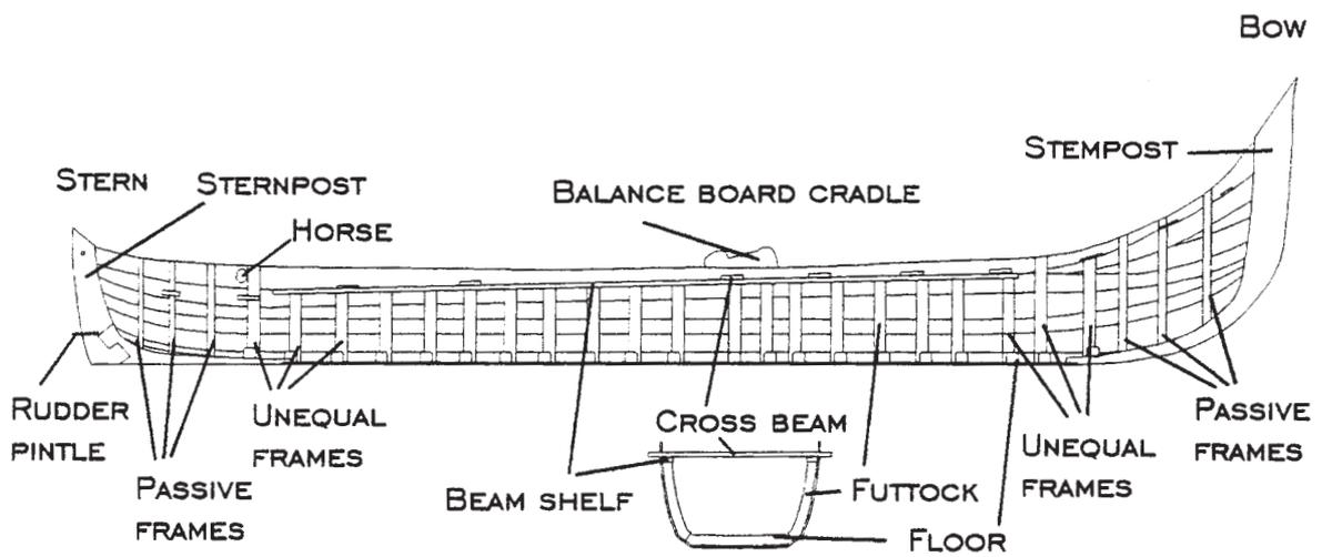
FIG. 7 – Terms used in the text to describe parts of the *vattai*. Drawing: E. Kentley.
