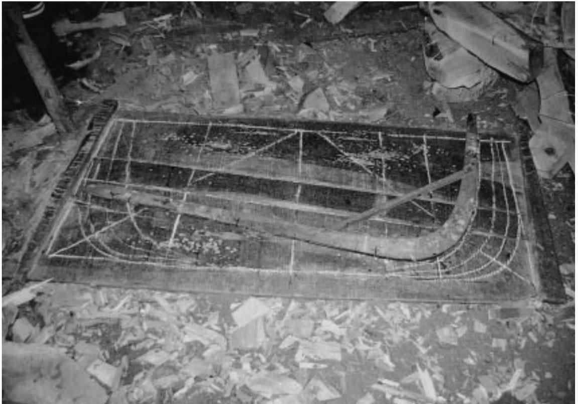
FIG. 8 – A scribe board and mould used in a boatbuilding shed at Atirampattinam. The preparatory lines and the shapes of the master frame and the three unequal frames have been highlighted in chalk. The angled parallel lines are not part of the design system, but merely outline one of the pieces of wood used to make the board. Photo: S. McGrail.
