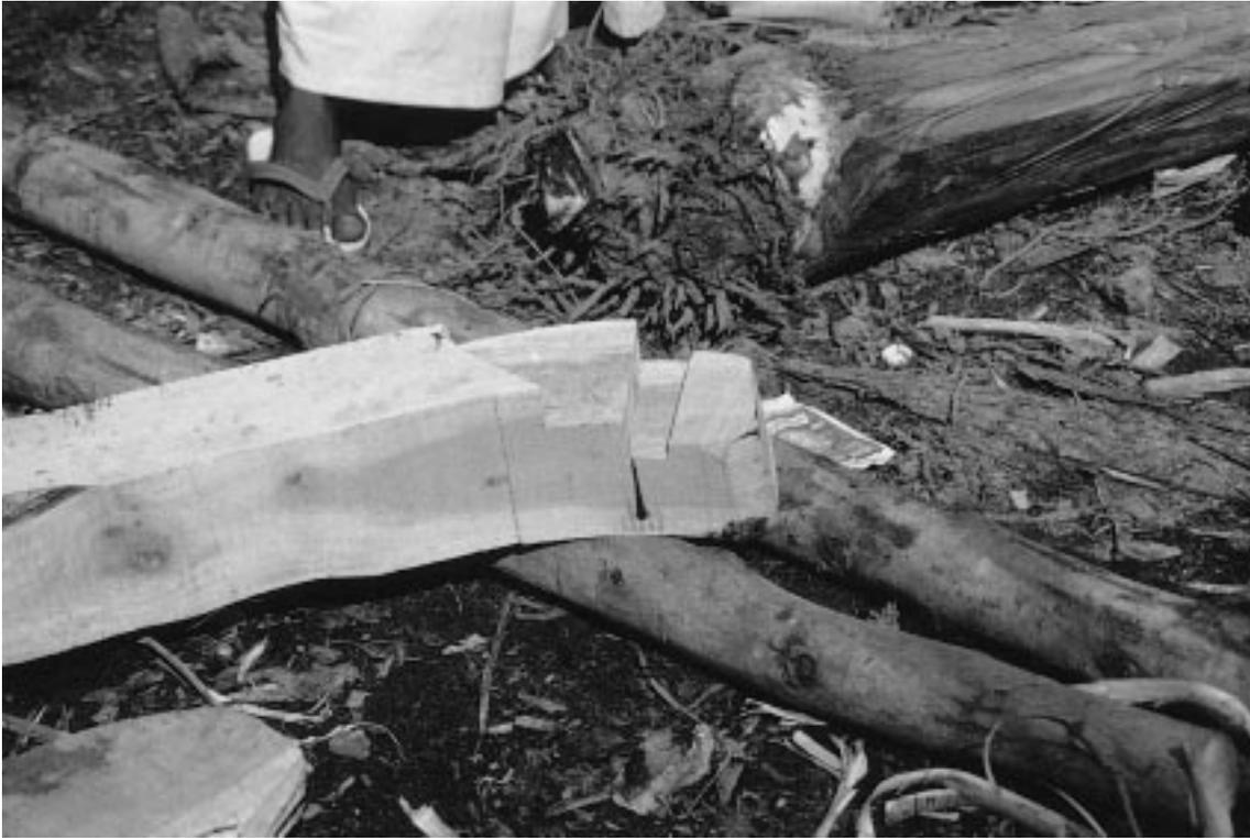
FIG. 10 – A *vattai* floor timber showing the futtock scarf. Photo: S. McGrail.
