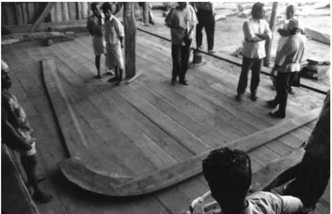
FIG.5 – A *thoni* two-part mould on a lofting floor in Tuticorin. Photo: S. McGrail.
