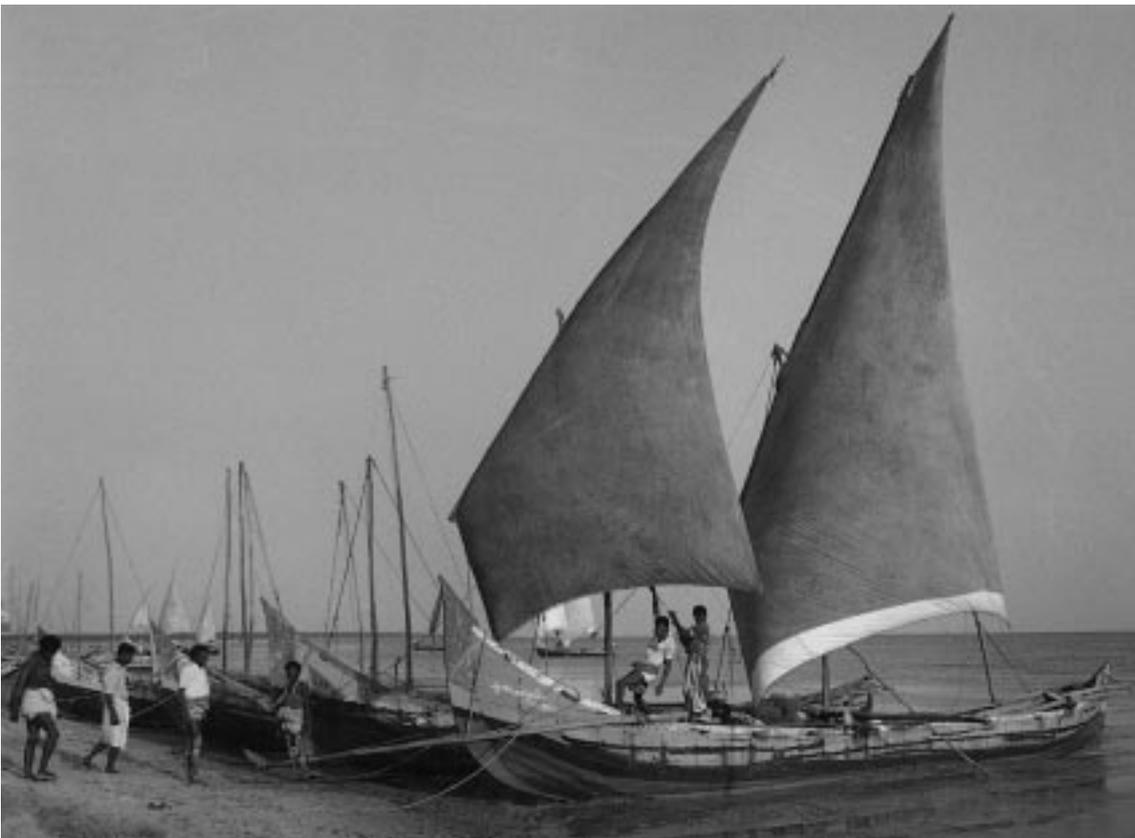
FIG. 3 – A *vattai* under foresail & mainsail taking the ground at the beach landing place at Eripurakarai, near Atirampattinam. Photo: E. Kentley
