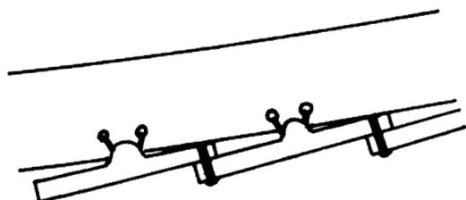
FIG. 3B – The planking laps, cleats, and frame lashing system of the Oslo vessels.
