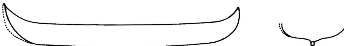
FIG. 3A – A sketch of the sheer and body shapes of a Viking vessel.
