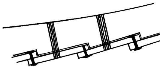
FIG. 3C – The notched frames and trenail fastenings of a Roskilde vessel.
