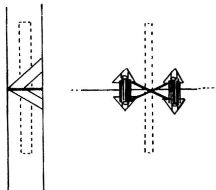
FIG. 2C – Edge and inner views of the sixth-century longitudinal seam lashing holes and one of the transverse aligning treenails (in dashed lines).
