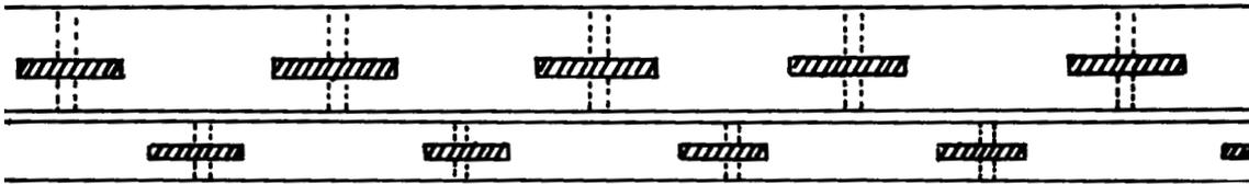
FIG. 2E – The Roman arrangement of edge-joinery in large double-planked hulls.
