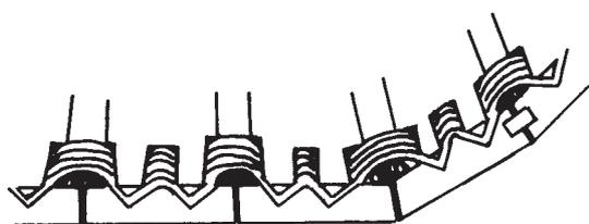
FIG. 2A – An edge view of the belts of transverse lashing on the Cheops hull.
