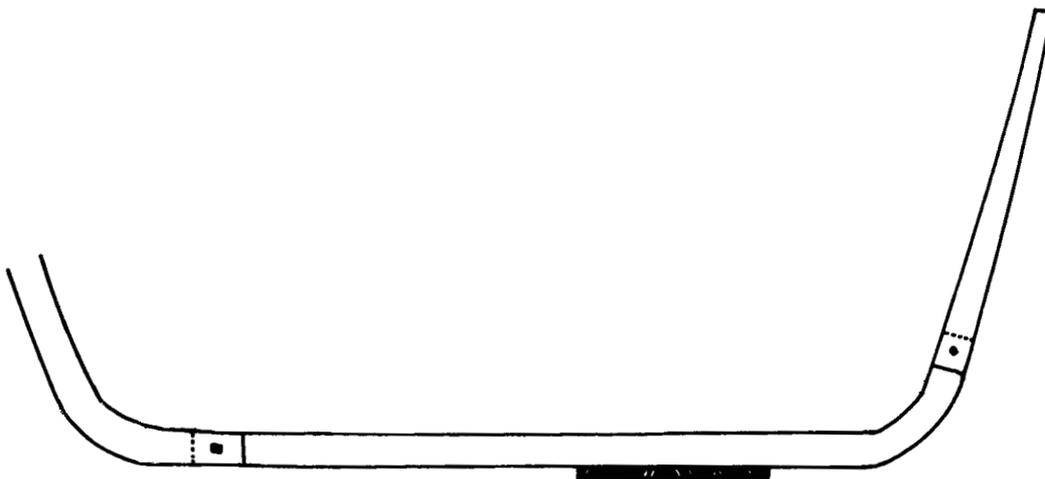
FIG. 2H – A pre-erected frames central frame in the Serçe Limani eleventh-century vessel.
