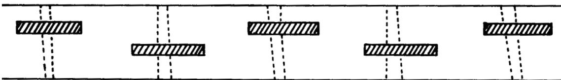
FIG. 2F – The Roman arrangement of edge-joinery in large single-planked hulls.
