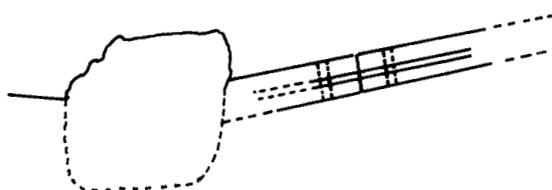
FIG. 2B – An *Uluburun* planking seam, mortise-and-tenon joint, and part of the keel.
