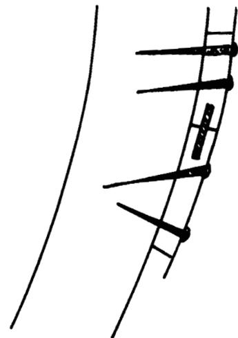
FIG. 2G – Planking seam alignment and nailing method of the Yassiada Byzantine vessel.
