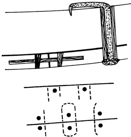
FIG. 2D – Edge and inner surface views of the mortise-and-tenon joinery systems and a typical clenched nail in The Kyrenia ship.
